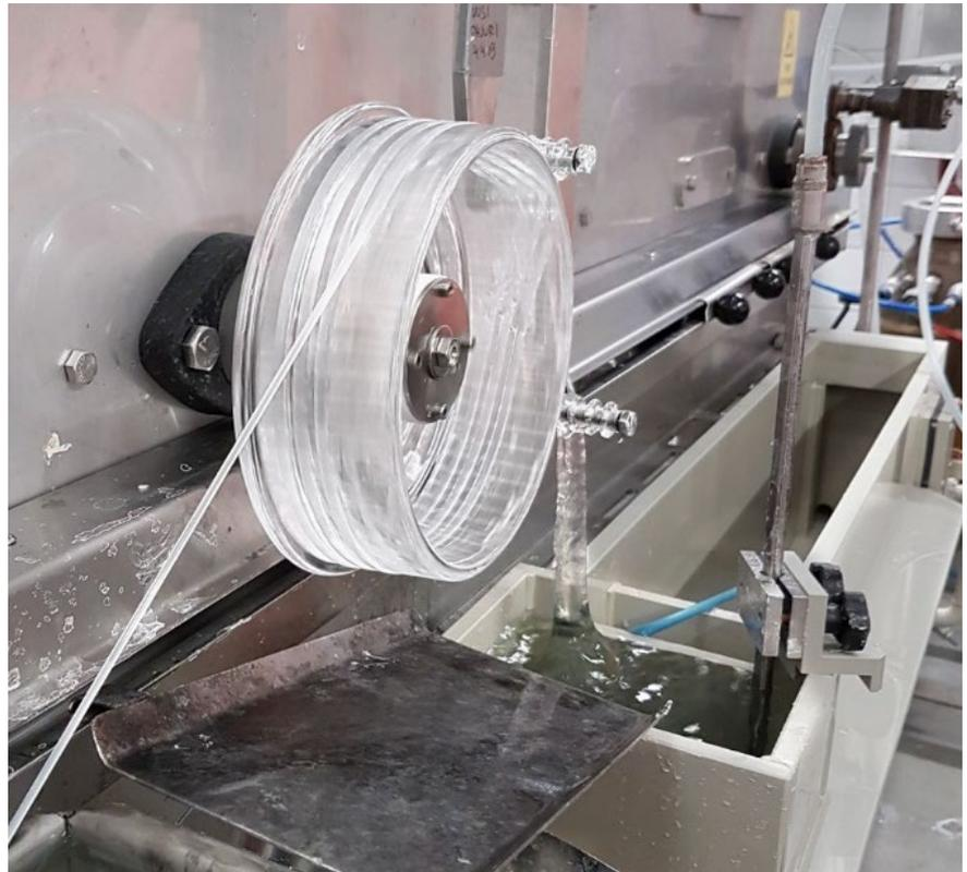
Picture from the VTT lab in Espoo, Finland. The as-spun fibre bundle with two thousand filaments is rolled up on the first godet.
