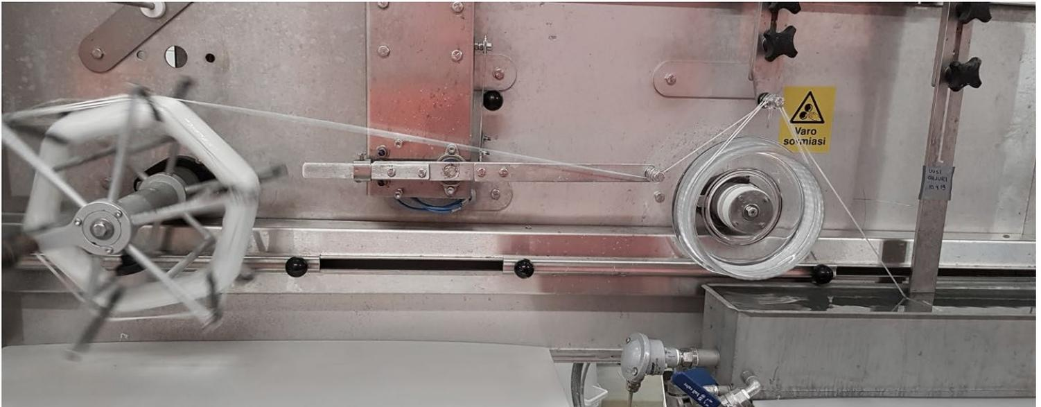
*From the final washing bath, the multifilament fibre runs two rounds on the last godet before it is wound up on the collector.*
